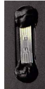
Figure 1 Flush mounted die on a ceramic substrate with glob top encapsulant covering the bonding wires
